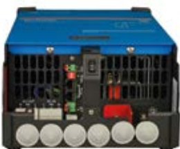
MultiPlus 2000 VA (bottom cover removed)
